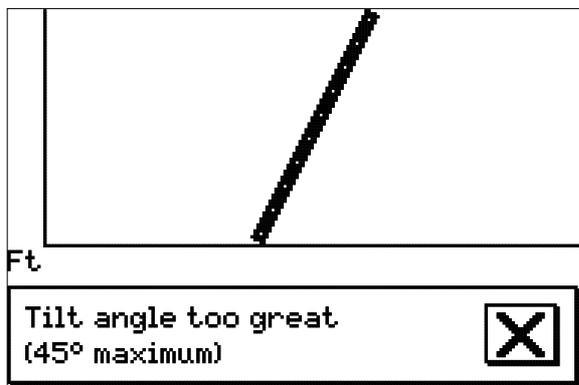
If the PPL Bar is tilted at an angle of more than 45° the 'Tilt angle too great (45° maximum)' screen is displayed.
